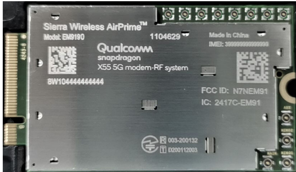
Figure 7-5: Unit Product Marking Example—Laser-etched, Typical Representation (Contents vary by SKU.)
